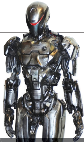
RAPID 2014 keynoter Jason Lopes from special effects studio Legacy Effects explained how he used Stratasys Objet Connex multi-material 3D printing to create the new RoboCop suit.
